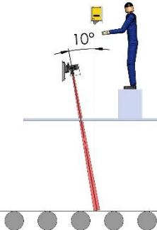
The back light **EMR-C** is installed below pass line, between 2 rolls.
