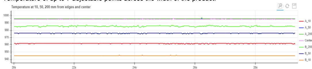
Specifications: 128 points per line, line period 25 ms, accuracy +/- 0.5% of reading plus +/- 3°C.
