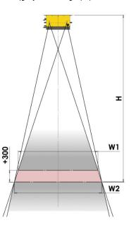
The accuracy in this table is given for a vertical field of 300 mm.
