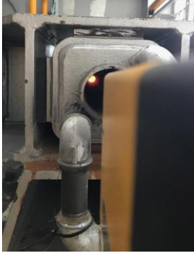
↪ Length & position measurement at furnace entry
