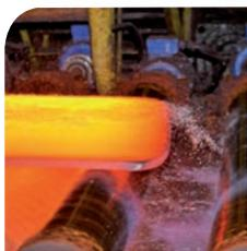
From the exit of reheat furnace to down coiler, DELTA hot metal detectors, infrared scanner and laser measuring sensors are extensively used for detection, edge positioning and measurement. They are able to work with high accuracy and reliability in the harsh environment of hot mills: high ambient temperature, heat radiation, steam, water, dust...
