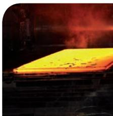
The ability to precisely measure the strip and plate dimensions during the hot rolling process is essential for the production of high quality steel and for achieving an optimum yield. DELTA has developed a range of measurement systems for installation in the extreme environmental conditions of the metal industry using the latest technologies with high resolution and high speed digital cameras.
