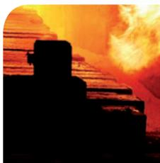
Typical applications in slab reheat furnace include detection, positioning and measurement of slabs on the charging table. DELTA sensors are able to work even on the very rough surface of slabs and to survive to the vibration and the heat especially in case of hot charging. DELTA has also developed some unique sensors for detection of slabs inside reheat furnace and at discharging side.
