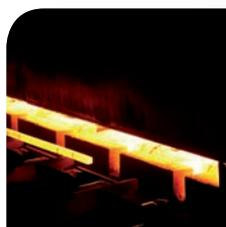
The charging operation is critical. It is important before moving the billet or bloom into the furnace to know the length and the position of the head and tail in order to avoid any damage.
