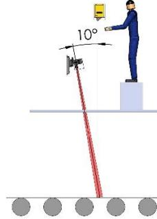
The back light **EMR-C** is installed below pass line, between 2 rolls.
